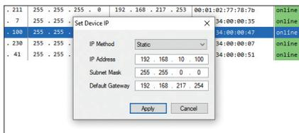
7 To access and configure the XVC-HEVC using the web-based user interface, enter the IP address of the encoder unit in the address bar of the browser.
